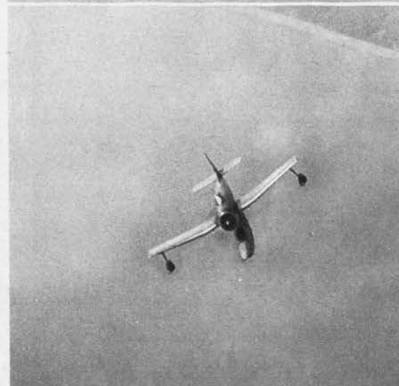
In all views, the Sea Hawk retains its distinctive appearance. Its head-on and overhead resemblance to the F6F is offset by a large single-strut float, tail fairing and cockpit blister.
